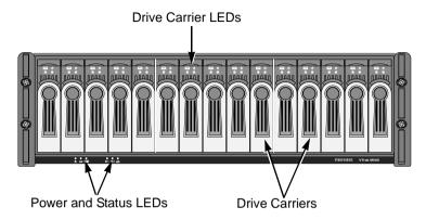
Figure 1. VTrak M500f/i/p front view
